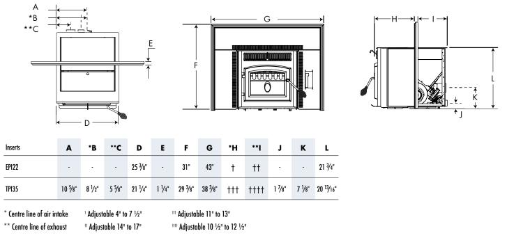
Measurements to be used as a guide only. Consult your owner's manual for complete and up-to-date installation instructions and proper clearances.
