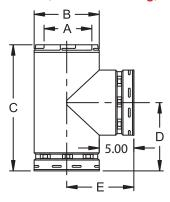
Note: Insulated Tee – 10"- 12" galvanized casing only. 14", 16", and 18" components are intended for use on chimney extensions only.
