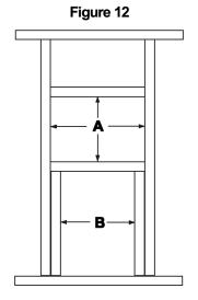
After framing in your opening to the dimensions specified to the Framing Tables 1 or 3, install the outer half (with the unfinished square plate) of the wall thimble into the outside wall opening. Secure in place using appropriate fasteners through the prepunched holes.
