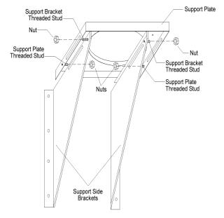
**Underside View of Threaded Studs and Nuts**
