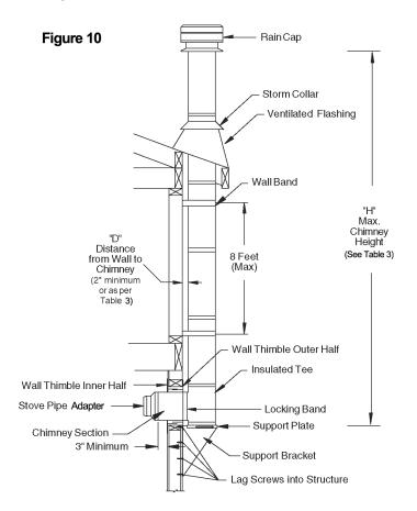
See Table 3 for maximum chimney heights based on chimney diameter and distance from wall.
