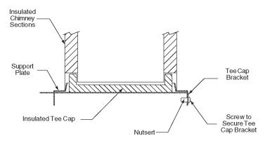
Securing of Insulated Tee Cap
