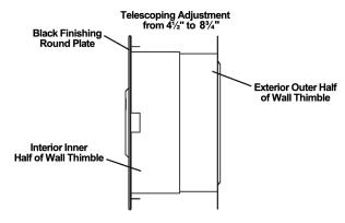
4. Install the inner half (with round plate) of the wall thimble into the inside wall opening, ensuring that the shield slides over the shield of the outer half. Once in place and flush against the wall, install the black finishing trim plate onto the wall surface and fasten in place with appropriate fasteners through the four prepunched holes.
