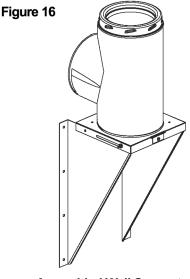
Assembled Wall Support with Tee Cap Secured in Place
