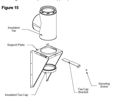
Explosion View - Wall Support, Insulated Tee and Tee Cap, Tee Cap Bracket, and securing Screw
