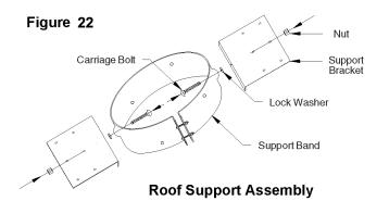
Slide the roof support down over the chimney section until its brackets rest on the roof or floor. Tighten the collar around the chimney with the nuts and bolts supplied, then secure the collar by screwing the six supplied sheet metal screws through the holes in the collar and into the chimney.
