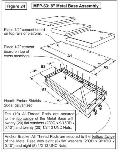
A IMPORTANT: Remember to tighten up nuts below the floor after fireplace installation in order to take up any slack in the threads.
