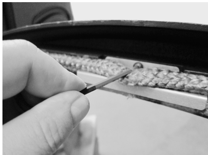
Figure 20. Loosen the glass clips.
