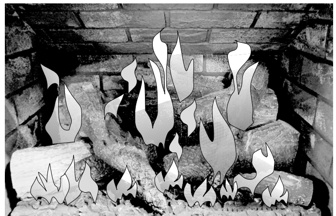
Figure 52. Steady state flame pattern - High setting.
