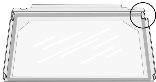
Figure 54. Bend the retainer tabs back enough to release the glass panel.
