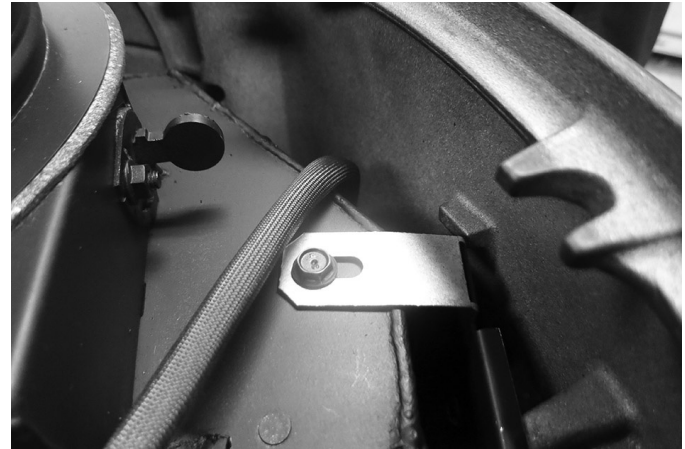
Figure 16.2. Remove the firebox-to-side plate bolt.
