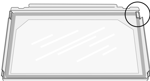
Figure 16.3. Bend retainer tabs only enough to remove the glass panel.
