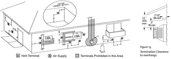
Figure 12. Vent Terminal Clearances - ANSI Z21.88-2014, CSA 2.33-2014, and National Fuel Gas Code.
