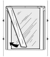
Figure 26a. Install Side Glass Panels.
