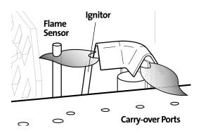
Figure 36. Correct Pilot flame pattern.
