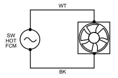
Figure 62. Wiring Diagram - GF 370 DV II Fan
