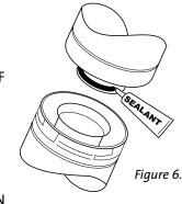
THE INNER AND OUTER PIPES. **DO NOT USE SILICONE.** SEE FIG. 6. SEE VENT MANUFACTURER'S INSTRUCTIONS.
