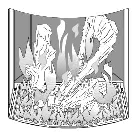
Figure 38. Proper flame picture -Traditional Logs.
