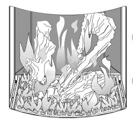
Figure 32. Correct Pilot flame pattern.
