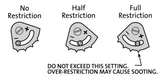
Figure 15. Exhaust Restrictor settings
