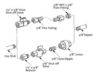
Figure 19. Gas supply valve types and fittings.
