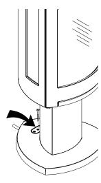
Figure 1. Pallet screw location
