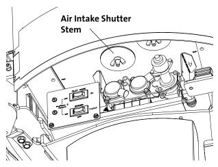
Figure 16. Air intake shutter location.
