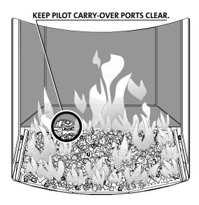
Figure 65. Starfire Glass flame picture.
