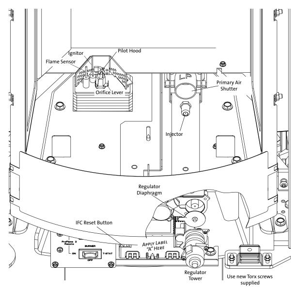
Figure 23. Fuel conversion components and assemblies
