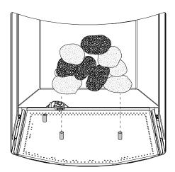
Figure 27. Set River Rock assembly on pins.
