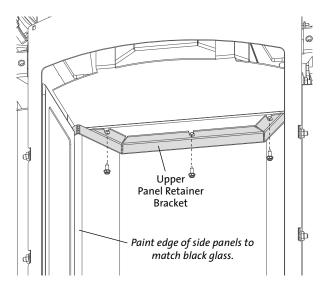
Figure 25. Loosen the panel retainer screws.
