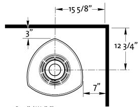
Figure 5. Parallel Wall Clearances.
