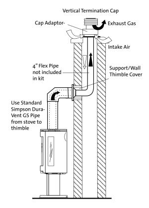
Figure 8. Approved masonry chimney conversion kits. A **Coaxial** chimney conversion system is available from M&G DuraVent, Pro Series® 46DV IIA-KMC and 6DV IIA-KCT. ICC, Inc. manufactures a Coaxial-to-Colinear adapter,
