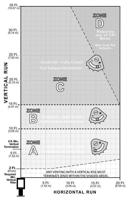
Figure 17. Vent Termination Diagram.
