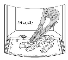
Figure 29. Lean the Right Log up against the upper right corner of the firebox and engage its toe with the indentation in the Bottom Log.
