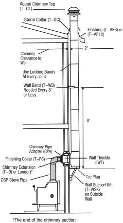
\*The end of the chimney section must extend into the room a minimum of 4–1/2" beyond the face of the wall.
